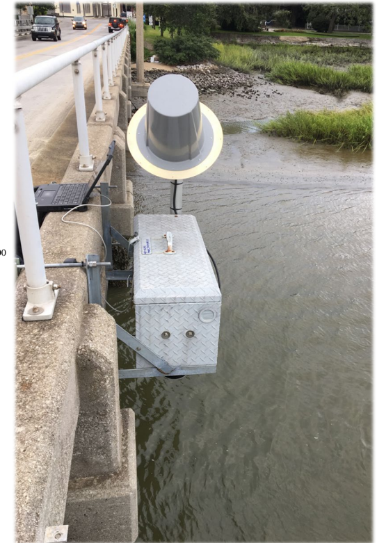
USGS rapid deployment gauge installed on US 21 bridge.
