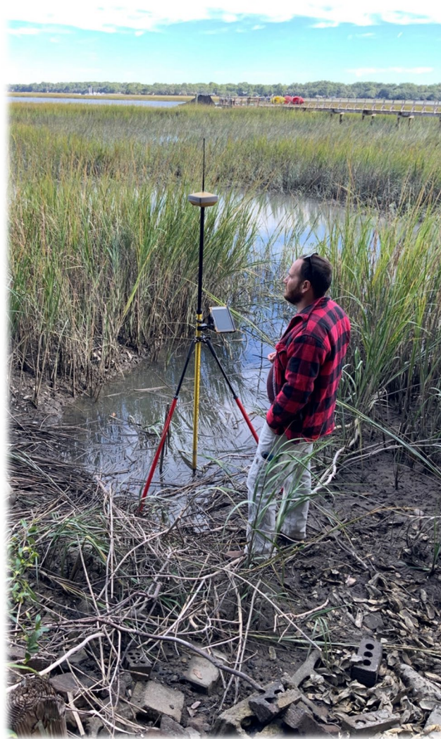
GPS survey at Pinckney Street/Bayard Street outfall.
